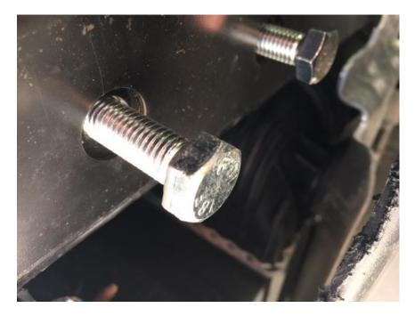
Remove front bolt and install tow hook on rear bolt.
